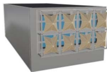
Figure 4. Facade Shading Element Based on the Opening and Closing of Purpurea Flower (Khelil et al., 2020)
